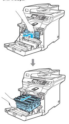
5 Release the gray lock lever (1) that is on the left side of the machine. Lift the front of the drum unit up and pull the drum unit completely out of the machine using the green handles on the drum unit.
